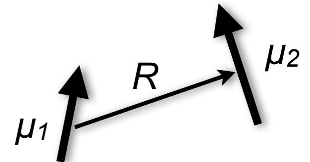
interaction energy of two dipoles  $\mu_B$  two Bohr radii  $a_0$  apart:
