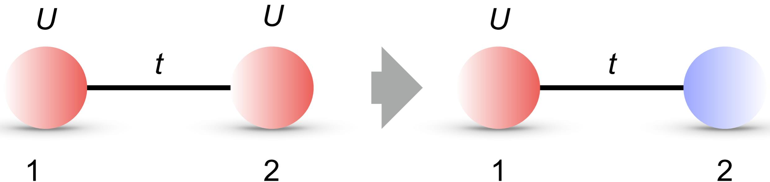
$$\hat{H} = \varepsilon_d \hat{n}_{1\sigma} + \varepsilon_s \hat{n}_{2\sigma} - t \sum_{\sigma} \left[ c_{1\sigma}^{\dagger} c_{2\sigma} + c_{2\sigma}^{\dagger} c_{1\sigma} \right] + U \hat{n}_{1\uparrow} \hat{n}_{1\downarrow}.$$
