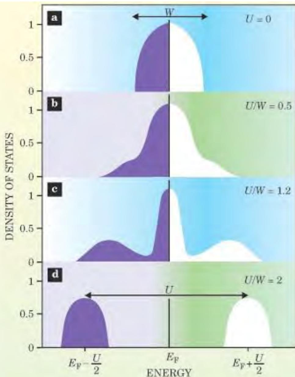
$$H = -t \sum_{\sigma} \sum_{\langle ii' \rangle} c_{i\sigma}^{\dagger} c_{i'\sigma} + \sum_i U n_{i\uparrow} n_{i\downarrow}$$
