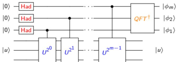
$$|\text{reg}\rangle = \frac{1}{\sqrt{2^m}} (|0\rangle + |1\rangle) (|0\rangle + |1\rangle) \dots (|0\rangle + |1\rangle) |u\rangle$$
