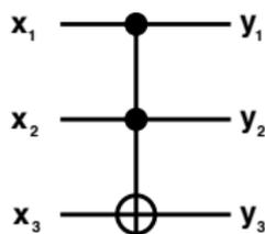
$$\begin{aligned} \text{AND : } & \text{ccNOT}(x_1, x_2, 0) = (x_1, x_2, x_1 \cdot x_2) \\ \text{cNOT : } & \text{ccNOT}(1, x_2, x_3) = (1, x_2, x_2 \oplus x_3) \end{aligned}$$
